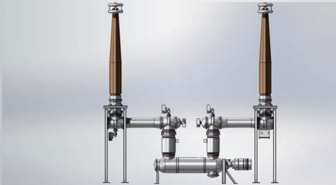
ZF15-550 HGIS ( with one circuit breaker ) structural layout
